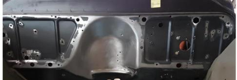
**6.**Take both passenger and driver fillers and transfer hood hinge hole location and brake booster location (If desired). Drill holes into the fillers for hood hinges. You can now place the hood hinge brace on both the inside driver and passenger side for re attachment. We suggest welding braces on.
