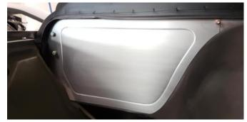
**3.** At this time please make reference to any factory bolt locations you wish to retain. Example: Hood Hinges and mounting brackets along the original firewall or brake booster. Write down the measurements for later reference. (Panels do not come with holes for cab and year diversity)
